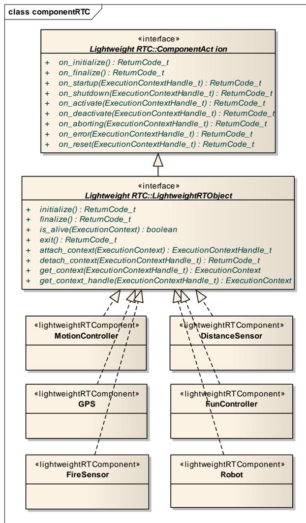
Figure 3. PSM of the Robot firefighter: Component's implementation.
