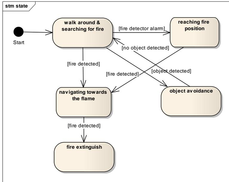
Figure 2. PIM of the robot firefighter: Behavioral Model.
