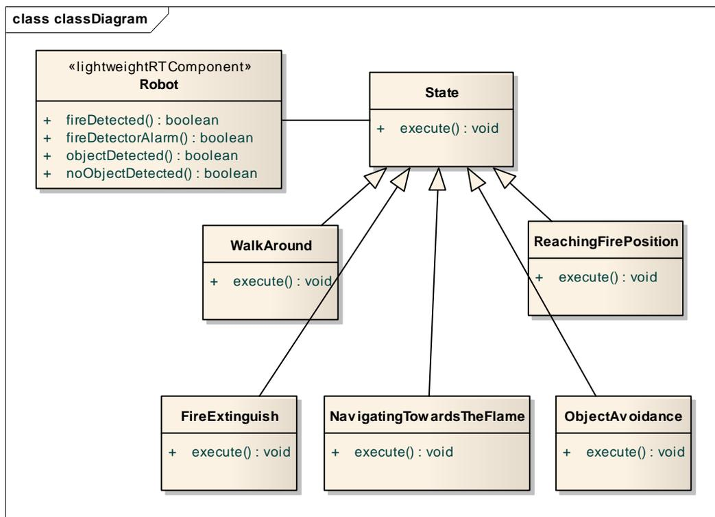
Figure 4. PSM of the Robot firefighter: Behavior's implementation.
