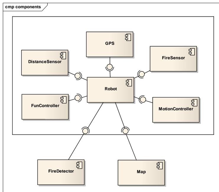
Figure 1. PIM of the robot firefighter: Component Model.
